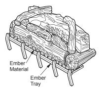
Figure 47 - Applying Ember Material
